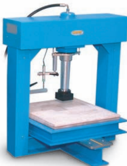
C090-14 + S336-14 fixed on the flexural machine C090-07N
