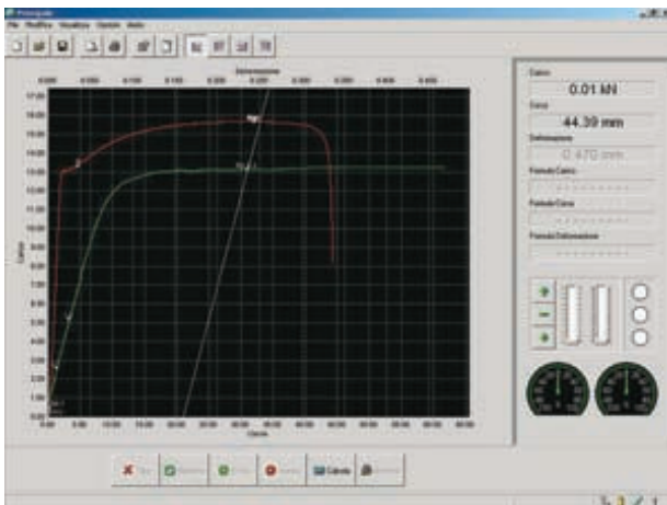
Tensile test on a steel specimen using tan extensometer, showing the symbols of the considered dimensions and the relative tracing in different colours selectable by the user.
