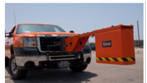
Vehicle-mounted RoadScan system integrated with FWD.
