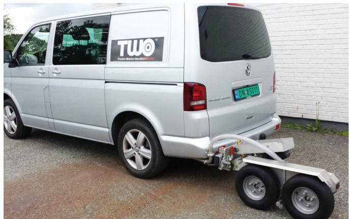
**Friction meter using precise weight values for definition of friction.
