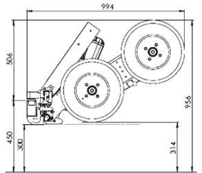
TWO is a vehicle-mounted gauge for effective measurement of friction on roads and airport runways. When used on the road, TWO is mounted on the left side of the vehicle, to measure the left wheel tracks and for airport the TWO is mounted so that the measuring wheel, detects the friction value between the tire and the runway in the center of the vehicle. The unit is raised and lowered by an actuator and controlled by the TWO software installed on the laptop inside the cockpit of the car.
