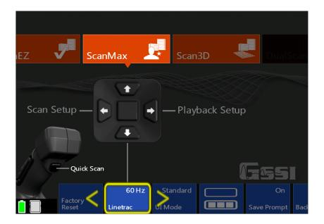
The StructureScan Mini XT comes equipped with the LineTrac XT software package. Simply insert the LineTrac XT into the front accessory port on the StructureScan Mini XT system. Select the LineTrac XT module and choose between 50 Hz or 60 Hz.
