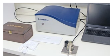
Above: TGA 4000 and DSC 4000 are both thermal analysis instruments from PerkinElmer. Below: TCi is a thermal conductivity meter from C-Therm Technologies.
