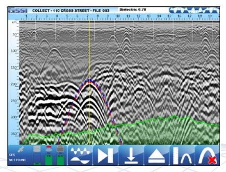
Data illustrates several metallic and non-metallic targets at various depths in blend mode. Green shaded area represents estimated signal floor. Red/blue dotted line identifies the soil velocity calculation tool.
