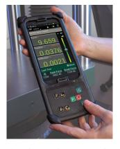
The Bluetooth connected interface features easy to operate tactile buttons and a high resolution touchscreen to set up and monitor tests where parameters and results are shown numerically. The interface also features an 8MP camera and has WiFi connectivity.
