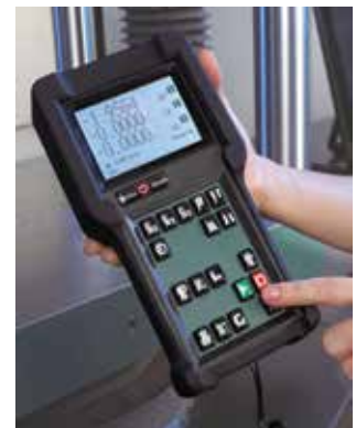
This tethered interface option features larger tactile feedback buttons for the operation of the testing frame; these make it ideal for users who need to wear protective gloves while operating the machine. The display provides simple numerical display of individual channels used on the testing machine.
