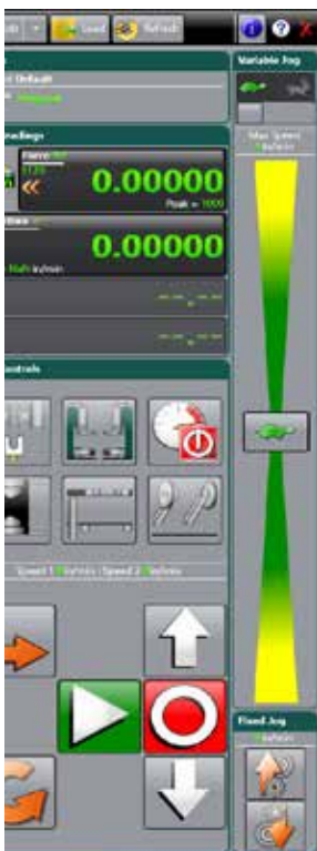
This virtual interface runs on a connected PC and can be used to set up and run a test to provide a quick numerical result. The addition of Horizon software with any of these interfaces allows complex tests to be created and recalled, along with sophisticated data analysis of all graphical data.
