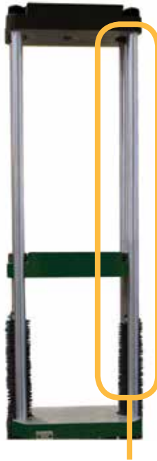
On this 150SL frame the columns have been extended to accommodate large test specimens.
