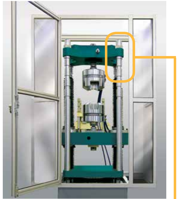
On this 600SL frame the columns have been extended while the screws for the adjustable crosshead are standard length. Additionally, the columns are notched to accommodate the adjustable top crosshead and the whole machine is surrounded by a fragmentation guard.
