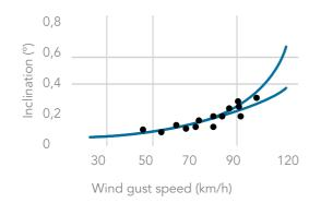
Exemplary diagram shows measured data points and wind tipping curve calculated from them
