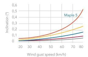
On the basis of the wind inclination curves, it is immediately apparent when a tree has an unusually high inclination value. As neighbouring trees are expected to have similar wind conditions, the high inclination value could indicate a less stability. The tree in question can then be examined more closely using the PiCUS Sonic Tomograph or another measuring method.
