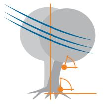
A base sensor measures the root plate inclination directly at the base of the trunk. A control sensor measures the inclination at a height of 2 to 3 metres so that the real wind reaction of the tree can be distinguished from sources of interference.
