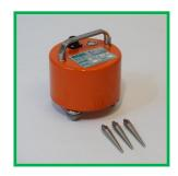
The 3D Land Geophone Mod. 3DLG-2 is the ideal accessory to add to your seismic instrumentation and perform HVSR, MASW and Vibration Analysis. One vertical and two horizontal high-performing sensors - with 2Hz resonance frequency and properly coupled - are mounted in a robust waterproof case, delivered with adjustable feet and interchangeable spikes.
