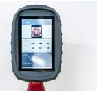
The working range of the instrument is  $0 - 2.000 \text{ cd x lx}^{-1} \text{ x m}^{-2}$ .
